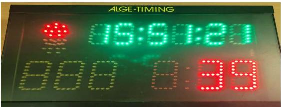
At 39 seconds from the start, a count is made from 39 seconds to 0, the light at the top left is in red
