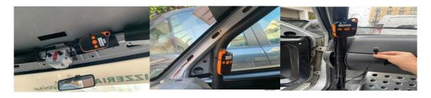
The GPS starts up when charging or with a long press of 5 seconds on the On/Off button located on the right side of the box (fig 1) the box vibrates and the LEDs flash: it is OK.
